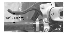
distance indicates low brake fluid level or air in the hydraulic system. Refer to the brake bleeding information on page 80.
